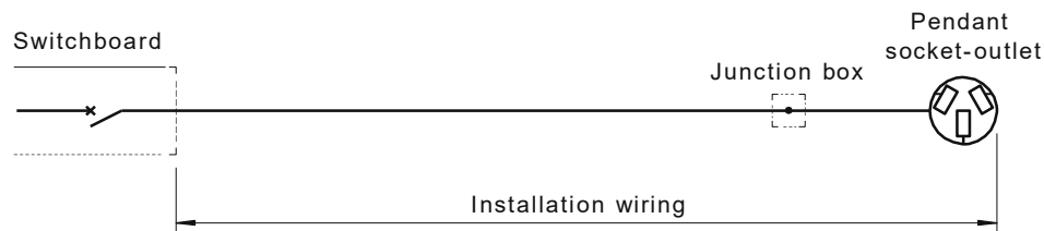
FIGURE 4.8 EQUIPMENT WIRING—EXCEPTION FOR PENDANT SOCKET-OUTLET
